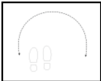
Figure 8. The 1236-X2 is balanced for sweeping in a tight semicircle. Always overlap your sweeps by at least 50% or you'll miss a lot of the deeper targets
