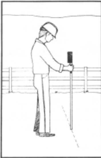
Figure 6. Vertical Position -Used for searching at high sensitivity levels and precise pinpointing.
